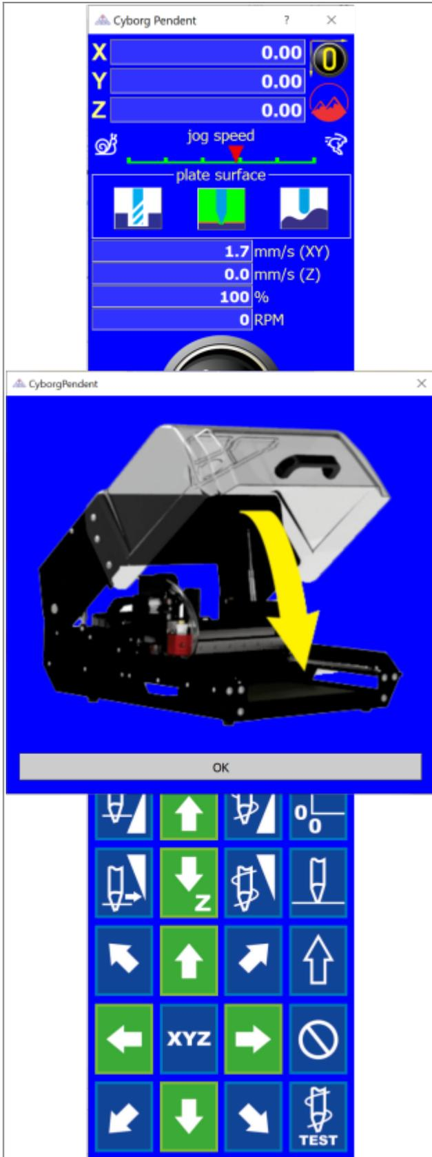
Before you can actually use the machine to engrave you will have to home it. In other words the machine has to find its limits and position itself over the top left corner of the engraving table. That is where the home position is. The home position is indicated with the coordinates (0,0).
