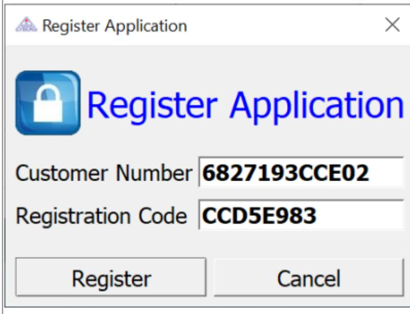
When the ethernet connection between your pc and the Cyborg X-300 has been configured correctly and the Cyborg X-300 has been switched on, then the registration window will display the machine's mac address in the "customer number" field. This is a unique code which is linked to the X-300 cnc controller.
