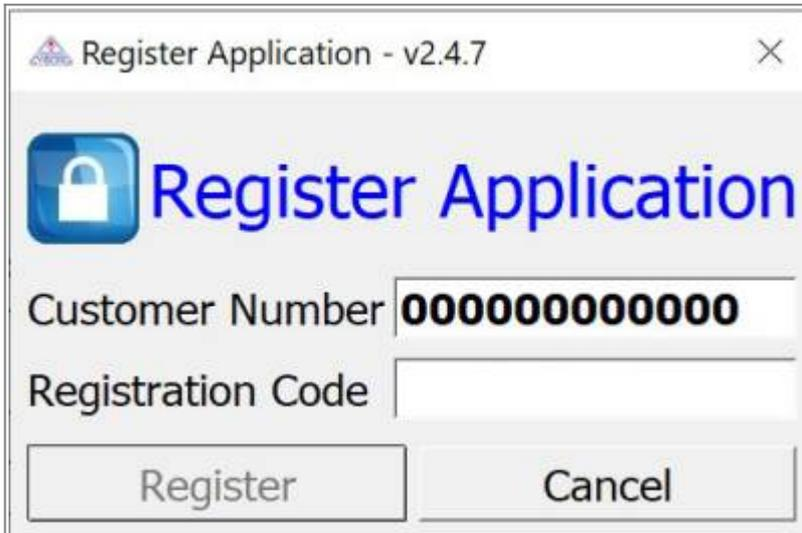
If a window such as the one here on the left appears then something is wrong with your ethernet connection, or with the ethernet cable, or the X-300 has not been switched on.
