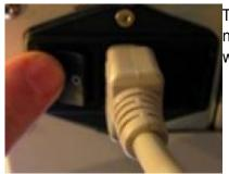
To switch on the power you toggle the rocker switch at the rear of the machine to the I position. (see image on the left.) It is not important in which order you switch on the machine and the program on the PC.
