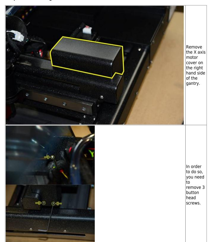
After removing those 3 button head screws, the X axis motor cover can easily be lifted.
