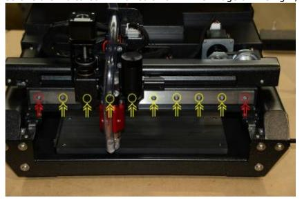
• You can then take the linear bearing with thespindle carriage in your hand and move them away from the gantry (see the image below). It is extremely important to hold the spindle carriage and the X axis linear bearing firmly in your hand and to make absolutely sure that the
