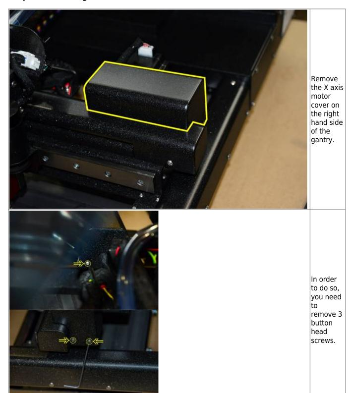
After removing those 3 button head screws, the X axis motor cover can easily be lifted.
