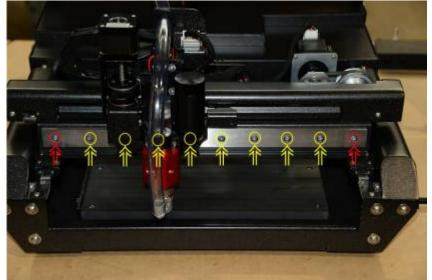
• You can then take the linear bearing with thespindle carriage in your hand and move them away from the gantry (see the image below). It is extremely important to hold the spindle carriage and the X axis linear bearing firmly in your hand and to make absolutely sure that the linear bearing cannot slide out of the bearing car, as it is almost impossible to slide it in again without sacrificing one or more bearing balls.
