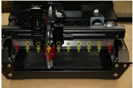
• You can then take the linear bearing with the spindle carriage in your hand and move them away from the gantry (see the image below). It is extremely important to hold the spindle carriage and the X axis linear bearing firmly in your hand and to make absolutely sure that the linear bearing cannot slide out of the bearing car, as it is almost impossible to slide it in again without sacrificing one or more bearing balls.
