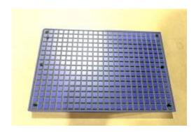
The optional vacuum table can replace the standard flat engraving table. It is supplied with spunge rubber cord to delimit the vacuum zone. under this phenolic table there is a compressed air connection. the vacuum hose goes from there to either a vacuum pump or a vacuum converter, both of which have to be provided by the customer (hense they are not included with the vacuum table). This vacuum table uses the same 6 screws which are used for the standard engraving table.
