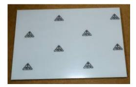
To secure the engraving material to this table you first have to put the sticky "Multimat" (standard included) on the engraving table. You then put the engraving material on the Multimat. The Multimat has 2 sticky sides. It will firmly hold the engraving material to the engraving table.
