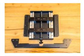
The centre vise can replace the standard flat engraving table. The standard engraving table has to be removed first, using 6 fixing screws, three on the left and 3 on the right of the table. The centre vise is fixed using the same screws. The standard front panel has to be removed (six screws and six washers). the special front panel can then be fixed to the chassis. This special front panel is visible on the picture, under the vise. The vise can be equipped with different clamping bars.
